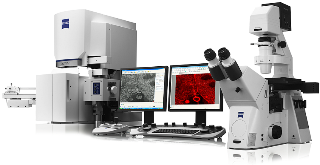
Fig. 28: SEM / LM system for correlative microscopy
